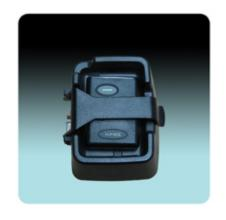
The *Unication NP88 Numeric Pager Programmer* includes programming software, a 4-pin programming fixture, a DB9 serial communications cable, and a 5VDC 1A power adapter. This fixture is unique to the NP88 pager.
