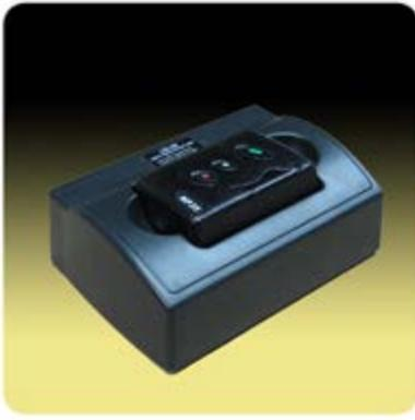
The **USAAlert NP35 Numeric Pager Programmer** consists of the programming fixture (labeled UB-08), the programming software (J8 for the NP35), and a USB cable for connection to the computer. The programming software is also used with the USAAlert Alpha 2 (J25) and NP40 (J7) pagers.
