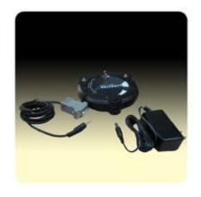
The *Unication Gearstar Pager Programmer* includes programming software, a coaster type programming fixture, a DB9 serial communications cable, and a 5VDC 1A power adapter.
