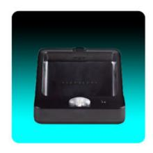
The *TPL Birdy WP Charger* Charger is an optional device if a rechargeable battery is preferred over the standard "AA" alkaline battery supplied with the WP pager. When charging, the pager will alert if receiving a message and a red LED indicator on the Charger will flash.
