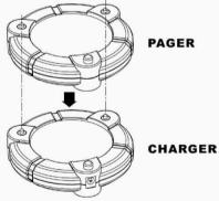
**Step4**: The pager power LED will go on when the pager is stacked correctly.
