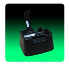
The *Unication Alpha Elegant Pager Programmer* includes a programming fixture, software, a DB9 serial cable, and a 5VDC 1A power adapter. The Alpha Elegant programming fixture is common for the entire line of Unication alphanumeric pagers and can be used interchangeably with Alpha Elite and Alpha Legend Plus pagers. The programming software is also common with the exception of the Alpha Elite pager that programs with its own software.
