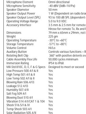
Omni directional 1 W (Dependent on radio brand/model) 93 to 100 dB SPL (dependent on radio brand/model) 3.5 mm & 2.5 mm for remote Rx audio or 6 pin Hirose for remote Tx, Rx and PTT functions 79 mm x 65mm x 29mm, not including belt clip Controls various functions - Radio and/or accessory related 360° with positive detents every 45°
